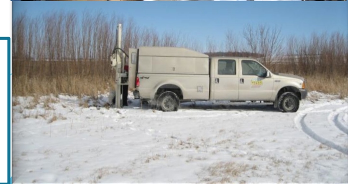
Iowa's hydro-geological ground water site assessment (Geo-Probe, mobile lab)
